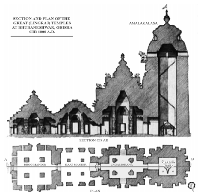
Fig. 2 Plan and section of Lingaraja Temple, Odisha, India [8, modified]
