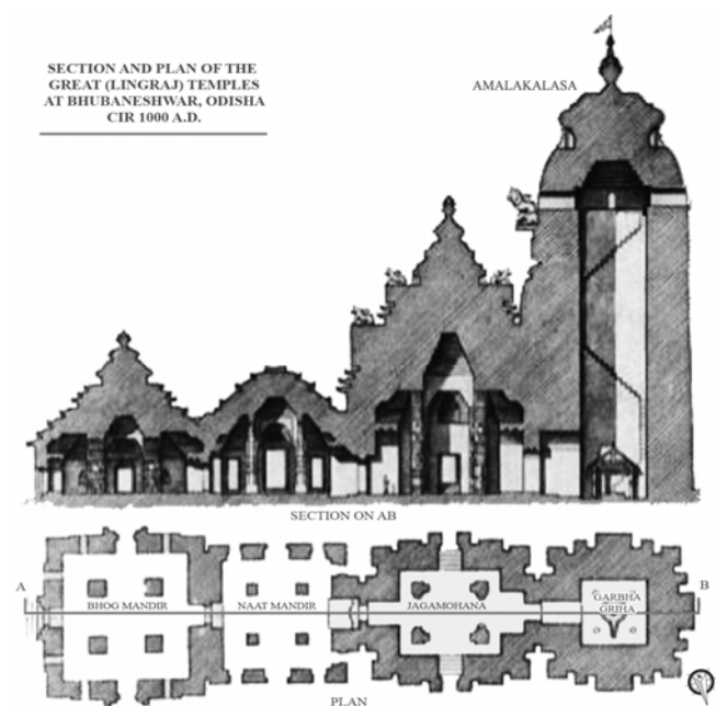
Fig. 2 Plan and section of Lingaraja Temple, Odisha, India [8, modified]
