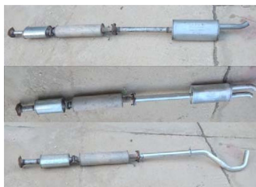
Fig. 2 Construction of the expansion chambers
