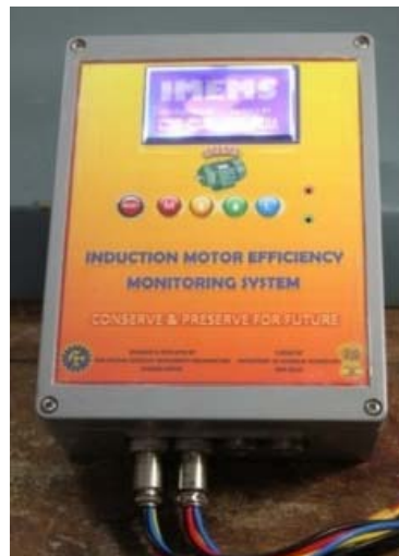
Fig. 3 View of the developed MPM Node
