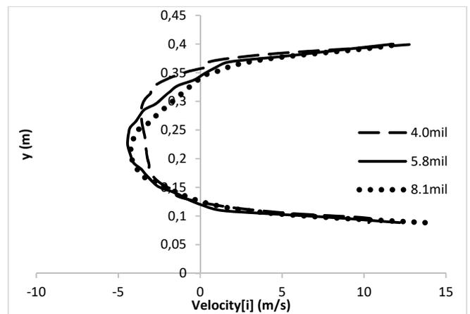
Fig. 6 Velocity profile obtained using three meshes
