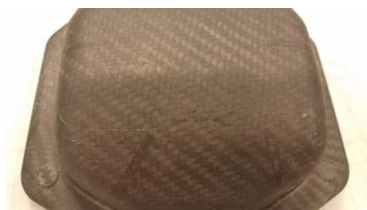
Fig. 9 Surface defects caused by mold surface cracking
