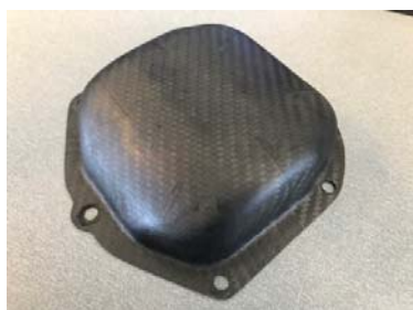
Fig. 7 Completed carbon fiber valve cover
