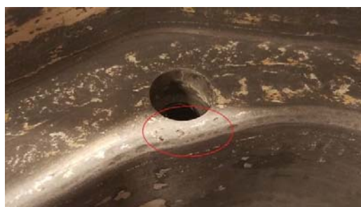
Fig. 10 Mold surface chipping
