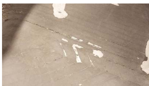
Fig. 11 Mold surface cracking between beads
