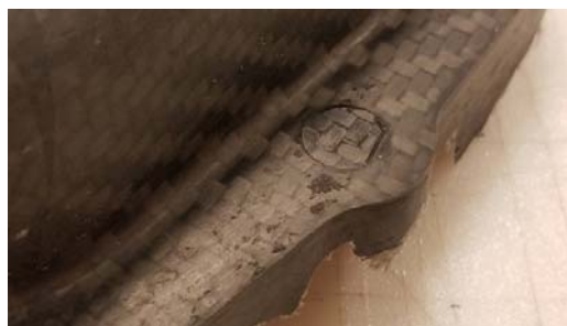
Fig. 8 Surface defects caused by mold surface chipping
