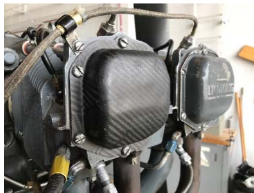
Fig. 14 Test fitting of carbon fiber valve cover
