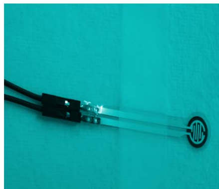
Fig. 1 A DF9-40 resistance type force sensor
