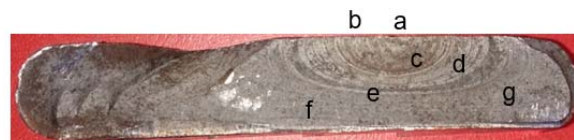
Fig. 6 Microscopic examination locations on the failed section
