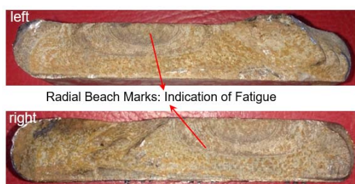
Fig. 2 Fracture surfaces at as-received condition
