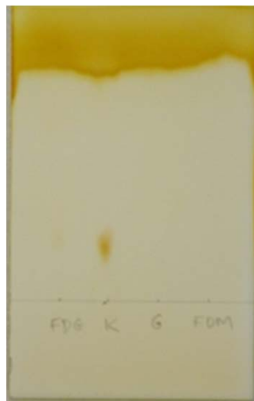
Fig. 2 Test for specificity of the method in the presence of possible components of ^{18}\text{F} -FDG (FDG: ^{18}\text{F} -FDG; K: kryptofix 222; G: glucose; FDM: fluorodeoxymannose)
