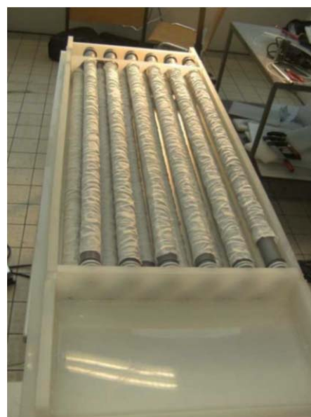
Fig. 3 PP tubes covered with textile sleeves
