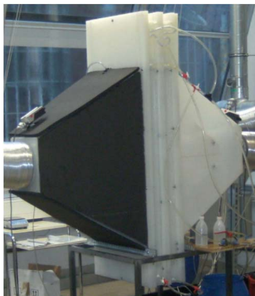
Fig. 4 Assembly of the absorber with air diffusers
