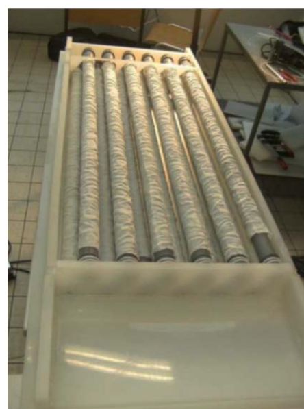
Fig. 3 PP tubes covered with textile sleeves
