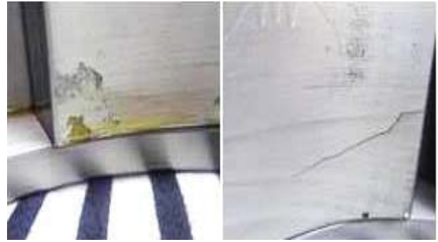
Fig. 8 Pitting and cracks on Babbitt layer of Bearing#01
