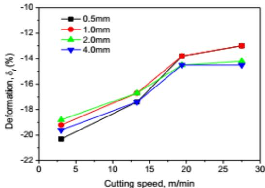
Fig. 7 Variation percentages of chips deformation along with the length with cutting speed at different depth of cut
