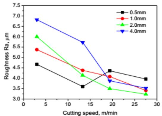
Fig. 2 Variation of surface roughness with cutting speed at different depth of cut
