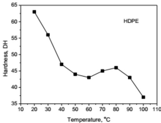
Fig. 4 Variation of hardness with real temperature
