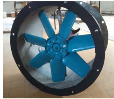
Fig. 3 Complete geometry of the counter-rotating rotor made
