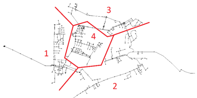
Fig. 8 The looping network split into four DMA regions using cluster analysis
