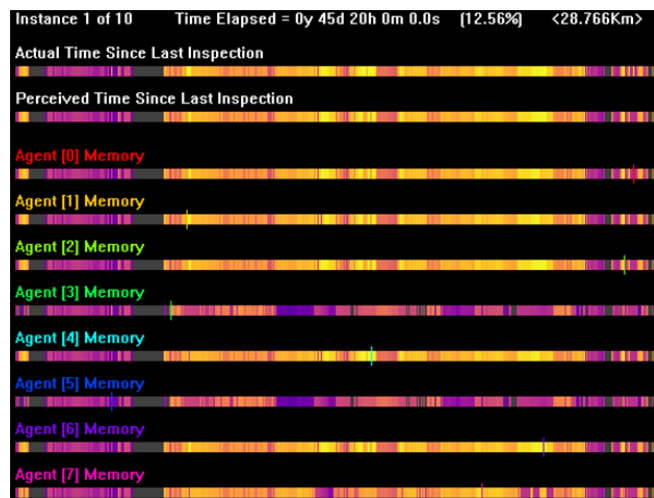
Fig. 7 Individual memories or 'maps' for each robot representing the Time Since Last Inspection
