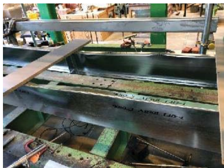
Fig. 6 Interaction bending/local buckling failures in BF-2
