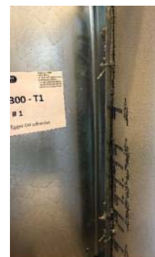
Fig. 5 Failure in specimens with screws and adhesive (P-300-A)
