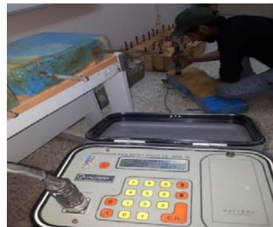
Fig. 10 Electrical resistivity measurement
