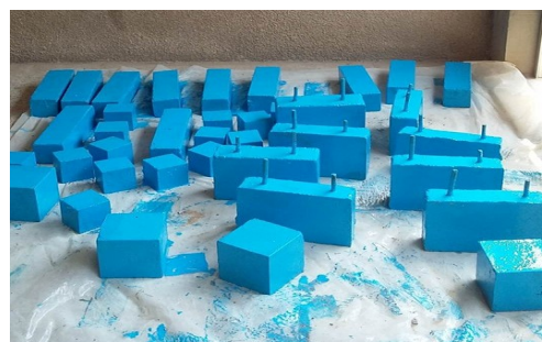
Fig. 2 Epoxy coating for the concrete specimens
