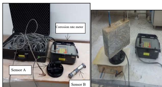
Fig. 4 Gecor 6 device and the setup of corrosion rate measurement
