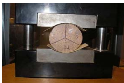
Fig. 3 Brazilian Test in laboratory
