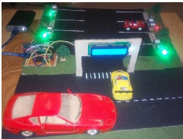
Fig. 17 L-IPS Working Prototype with Spot 3 in-use (1-Red LED); Spots 1, 2 and 4 available (3-Green LED)
