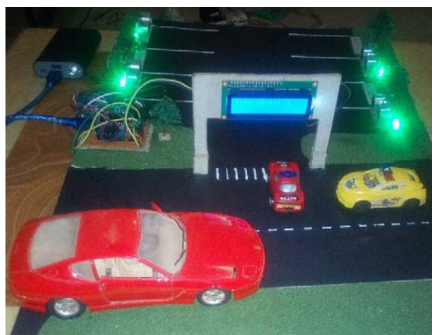
Fig. 16 L-IPS Working Prototype with Full (4) Parking Spots Availability (4-Green LED indicators)
