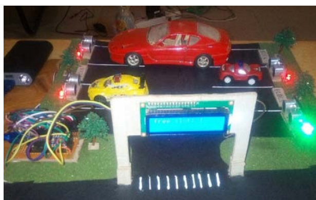
Fig. 19 L-IPS Working Prototype with Spots 1, 2 and 3 in-use (3-Red LED); Spot 4 available (1-Green LED)
