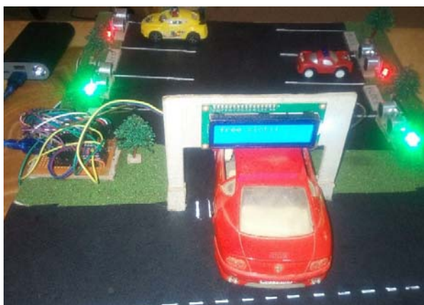
Fig. 18 L-IPS Working Prototype with Spots 2 and 3 in-use (2-Red LED); Spots 1 and 4 available (2-Green LED)
