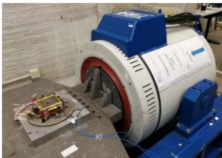
Fig. 6 DOC installed on the slip table for In Plane Test
