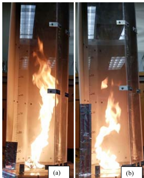
Fig. 3 Fire which was formed for cases with height factor of 1.36, (a) and, 3.18, (b)
