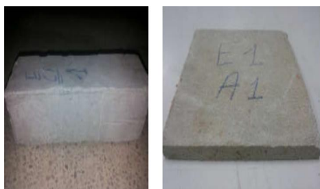
Fig. 1 Specimens made by addition of paper treated with cement and clay
