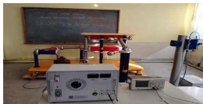
Fig. 7 200 kV lightning impulse voltage generator and water jet test system
