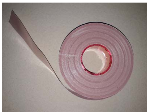
Fig. 2 Mica tape for VPI system
