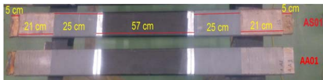
Fig. 3 Stator bar dimension
