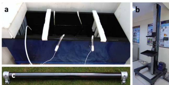
Fig. 5 (a) Chemical bath reactor (b) Dip coater and (c) ARCI's indigenously developed 1m receiver tube
