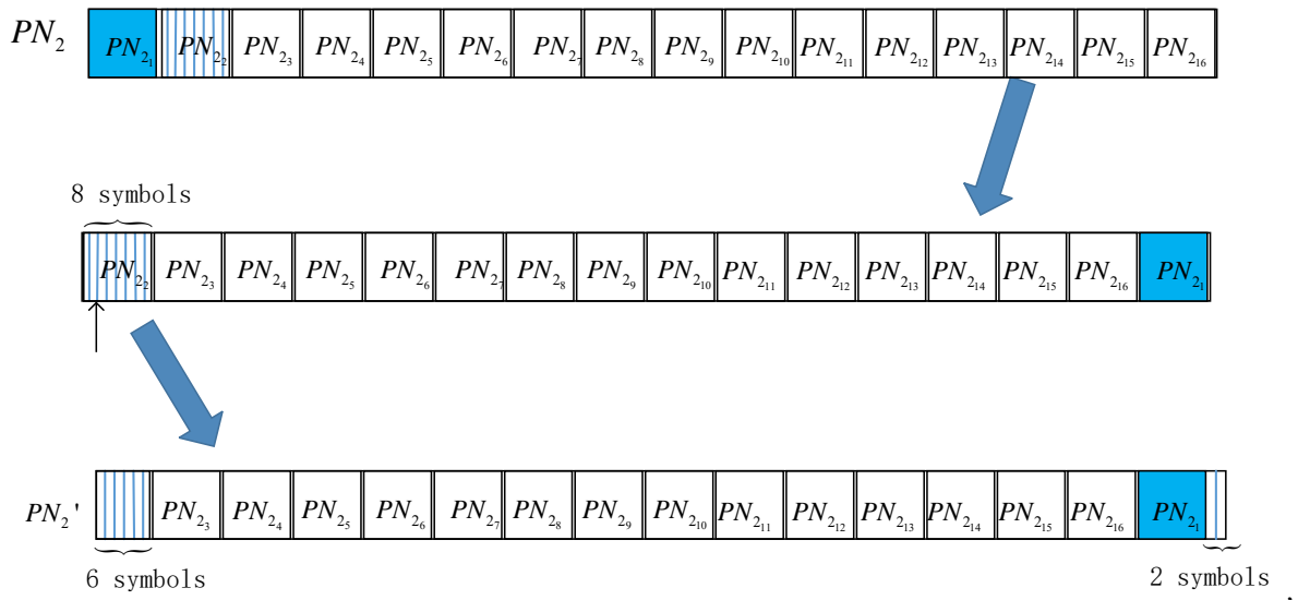
Fig. 3 PN_2 sequence cyclic shift diagram
