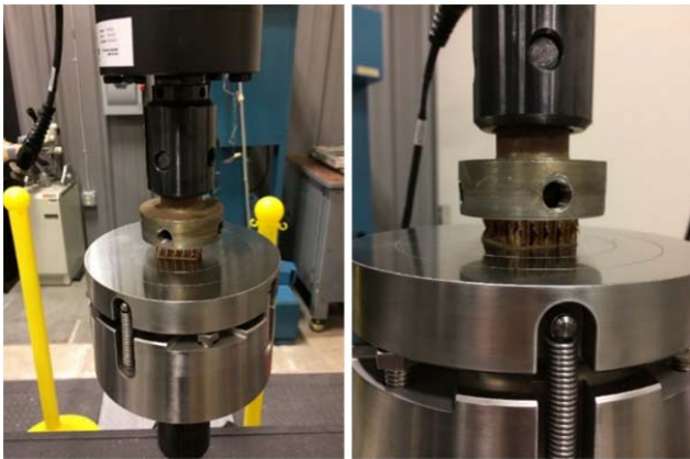
Fig. 2 Test Settings and the Compressed Test Specimen
