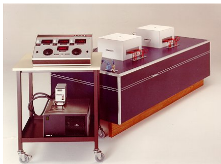
Fig. 3 Device for the measurement of thermal conductivity by the method of the box
