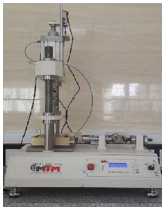
Fig. 3 Digital direct shear apparatus in IKIU lab
