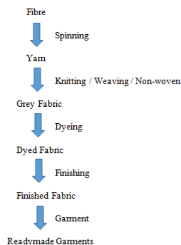
Fig. 1 Primary flow chart of a garment supply chain
