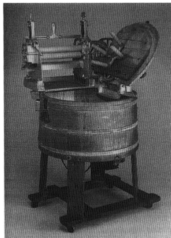
Fig. 1 Wooden domestic washing machine with a dolly-style agitator, 1920 [13]
