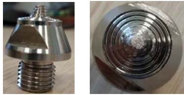
Fig. 17 A tapered circular with 3 flats pin used in this study
