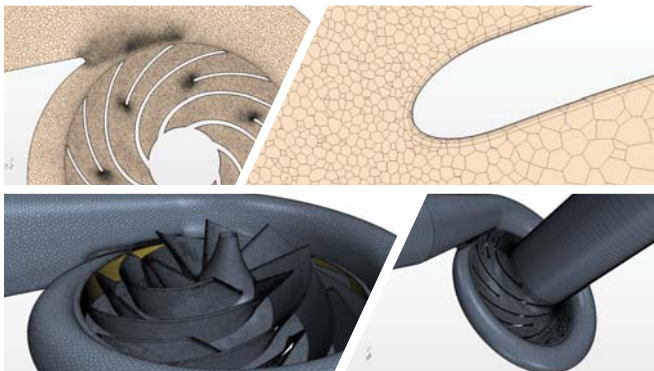
Fig. 7 Different views of reference compressor mesh
