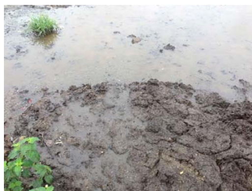
Fig. 3 (d) Concentrated household sewage sludge after dewatering
