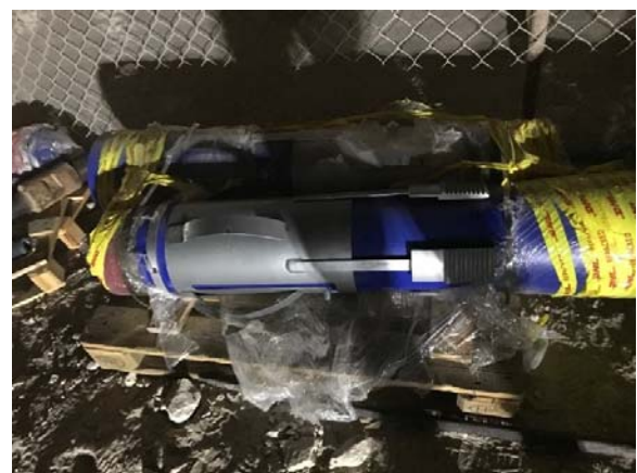
Fig. 13 Liner hanger used for extending the casing to 160 meters bgl
