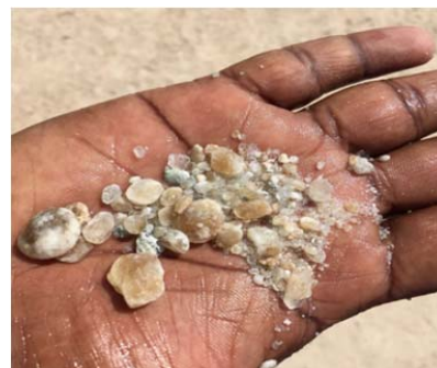
Fig. 6 Gypsum cuttings collected from drilling activities
