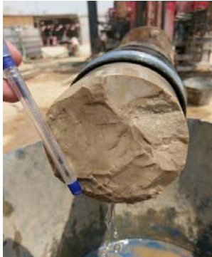
Fig. 7 Chert core sample from 77.95m bgl
