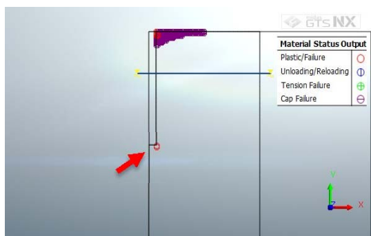
Fig. 27 Formed plastic points under load of 1500 kN
