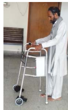
Fig. 11 Testing of gait trainer
