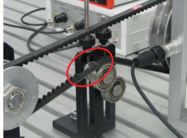
Fig. 2 Belt drive with Missing Cogs V-belt
