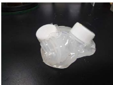
Fig. 1 Molten polypropylene bottles after heating
