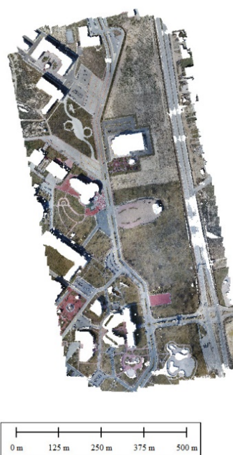
Fig. 3 Point cloud filtered by CSF (Ground point)
