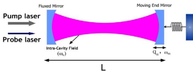
Fig. 1 Schematic model of Cavity-optomechanics. This model is the representative of the Cigar-shaped Fabry- Pérot cavity (length  $L$ ) optical system with one fixed mirror and one moving end mirror possess maximum amplitude of  $q_0$  driven by an external pump with frequency  $\omega_E$  and transverse probe field with frequency  $\omega_p$
