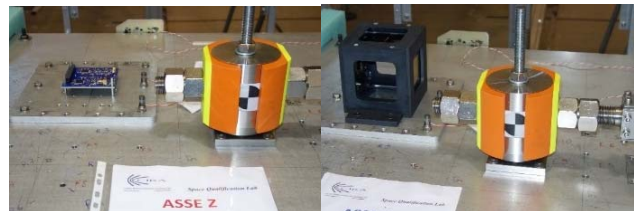
Fig. 13 CubeSat and modules installed on ringing plate of shock facility. Vertical axis
