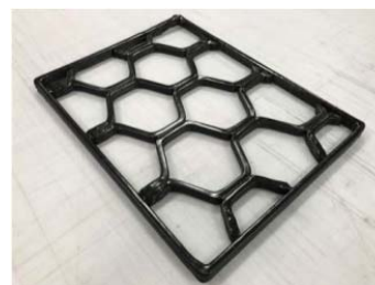
Fig. 1 Prototype 3D printed recycled carbon fiber part
