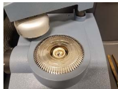
Fig. 8 Specimen loaded in DSC's chamber
