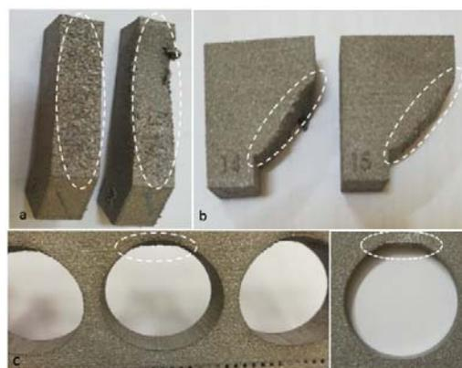
Fig. 13 Overhang structures distortions
