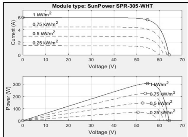
Fig. 5 PV Module Characteristics (I-V & P-V) Curves
