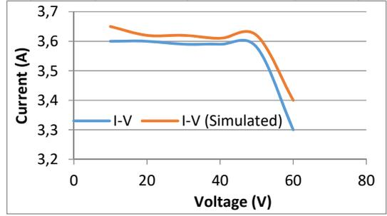
Fig. 7 Verification of PV cell (I-V curve)
