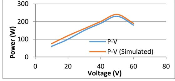
Fig. 8 Verification of PV cell (P-V curve)
