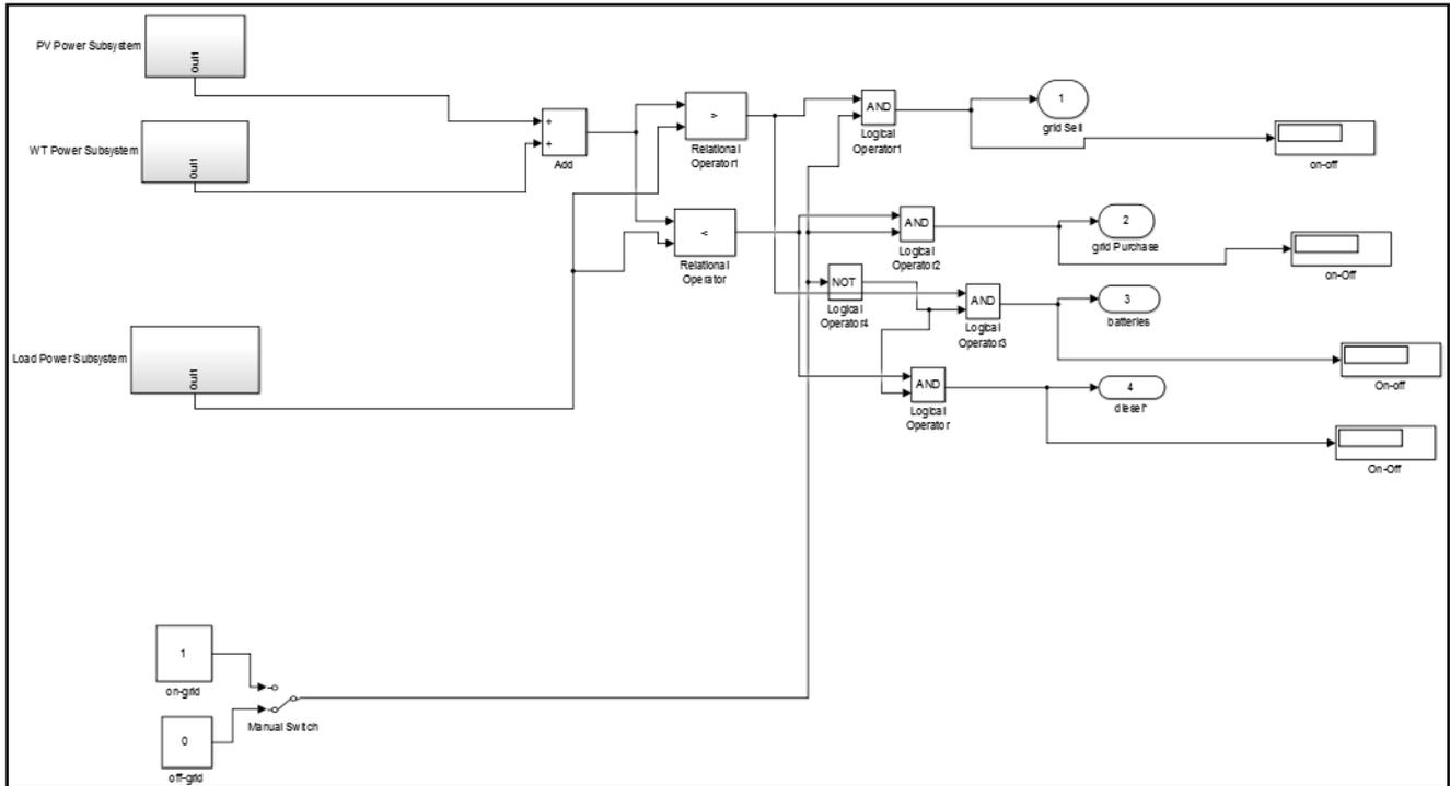
Fig. 2 Micro-Grid Control Model in MATLAB/Simulink (On/Off-grid mode)
