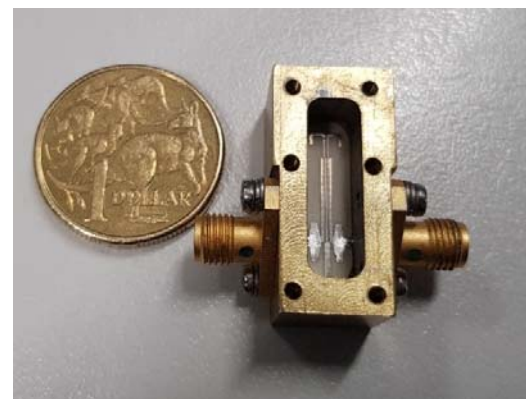
Fig. 3 (a) Fourth-order via less filter, and (b) fabricated prototype filter
