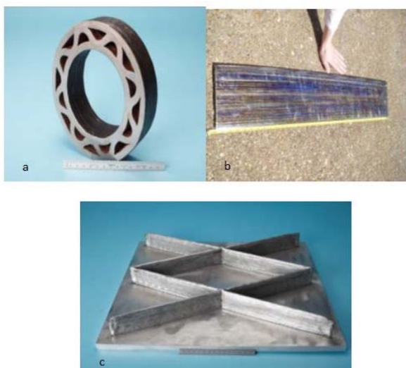
Fig. 5 WAAM components: (a) mild steel honeycomb structure; (b) aluminum stiffened Panel structure; (c) 1 meter long Ti64 wall structure [84]
