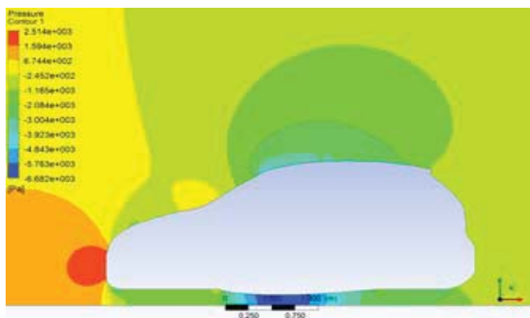
Fig. 19 Static pressure contour hatchback car body with an inverted airfoil of 1700 mm chord
