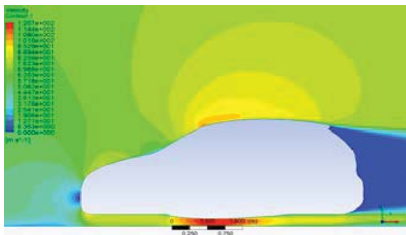
Fig. 20 Velocity contour of hatchback car body with an inverted airfoil of 1700 mm chord
