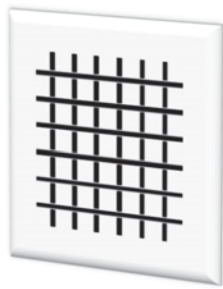
Fig. 12 Typical schematic turbulence grid used in experiments
