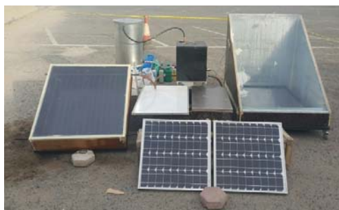
Fig. 2 Proposed solar desalination unit with preheater [9]
